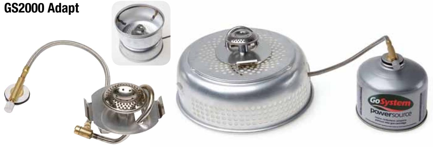
Designed specifically to clip into spirit non-pressured stoves, this unit will burn vapour or liquid gas due to its pre-heater tube (generator). It connects to a remote GoSystem EN417 gas cartridge through a braided hose and in conjunction with its precision flame control, has a performance way beyond its size. The unit packs away into the stove/cook set.
